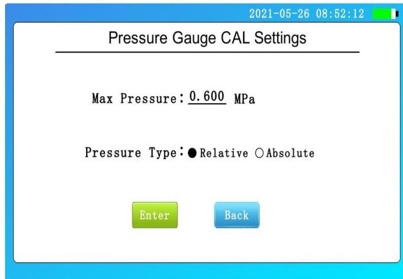
**Figure 3. 10 Pressure gauge calibration parameter setting interface**
