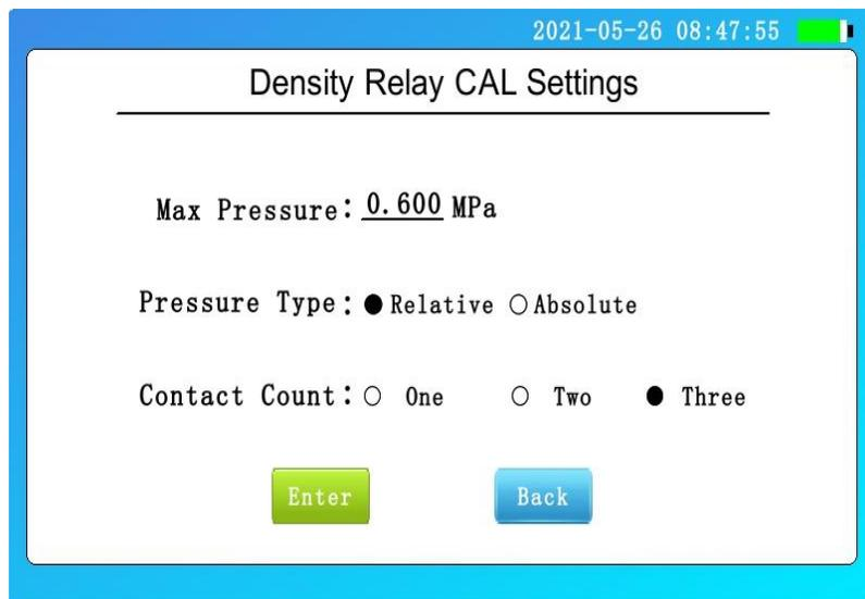
**Figure 3.2 SF<sub>6</sub> density relay calibration parameter setting interface**
