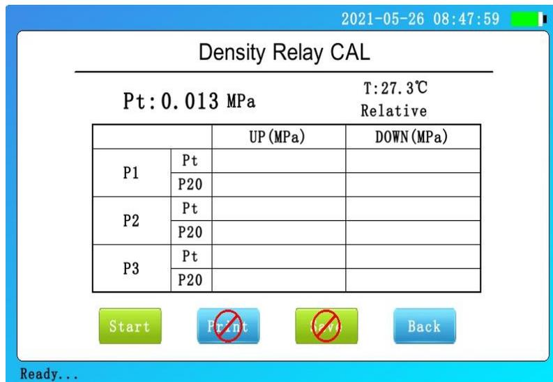
**Figure 3.3 SF<sub>6</sub> density relay calibration test interface**
