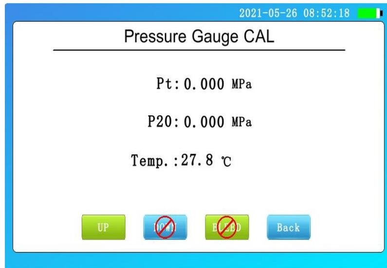
**Figure 3. 11 Pressure gauge calibration interface**
