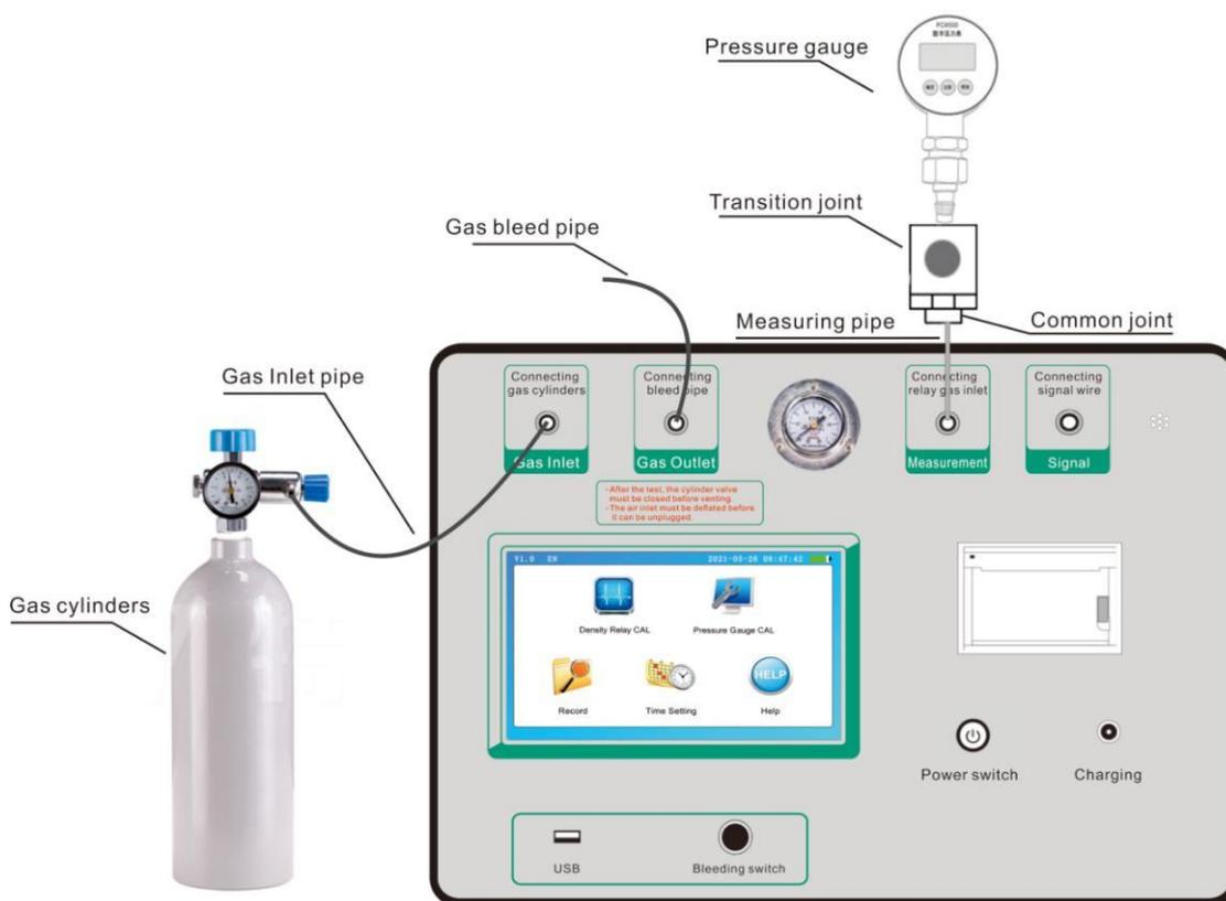
**Figure 3. 9 Calibration wiring diagram of pressure gauge**
