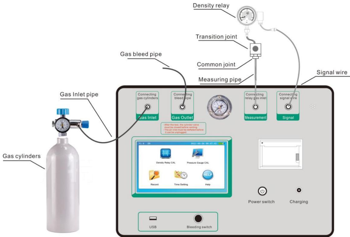
**Figure 3.1 Density relay calibration wiring diagram**
