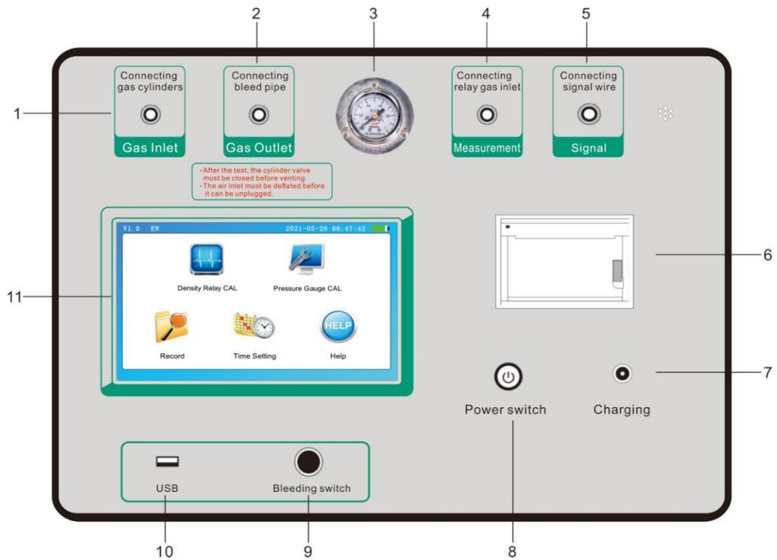
**Figure 1.1 Panel structure diagram**
