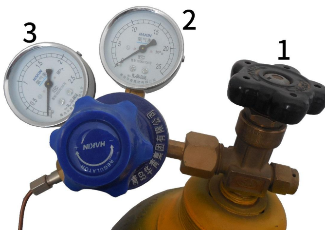
1.Total pressure valve 2. Total pressure gauge 3. Partial pressure gauge 0.4MPa Cylinder with pressure relief valve
