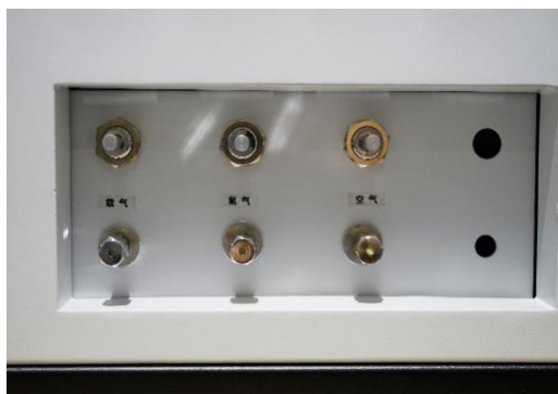
Figure 4 Figure 5(1 for carrier gas control switch ; 2 hydrogen control switch ; 3 air control switch) Where arrow thickness represents switch direction
