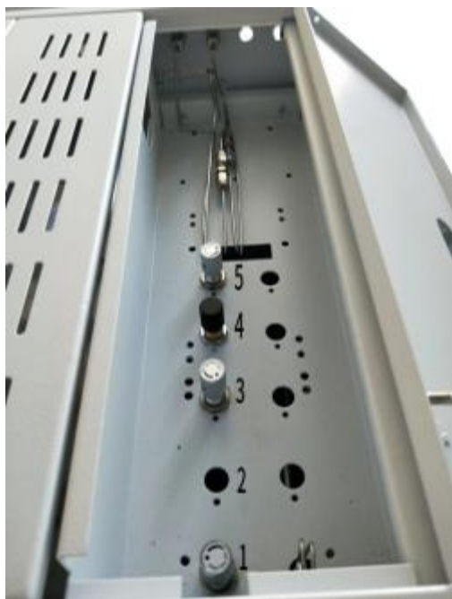
Figure 8 (Figures 1, 2, and 3 respectively show the carrier gas needle valve, hydrogen needle valve and air needle valve, 4 is a back pressure valve used to regulate the pressure in front of the column, 5 is a needle valve used to regulate the flow rate of the diaphragm)
