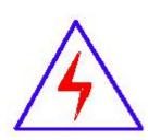
The input/output terminals and the test column may bring voltage, when you plug/draw the test wire or power outlet, they will cause electric spark. PLEASE
