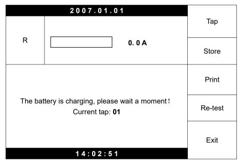
At this time, the current of the winding starts to increase. If the charging progress strip and the current display value stand still for a long time, it indicates that the value of the resistance value to be measured is probably beyond the measuring scope of the current, so it is not able to reach its set value. At this time, press "Exit" key-press to return and re-select the current and retry. When the set value is reached, it becomes constant. Then, enter into
