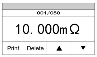
The upper part of the screen shows the total number of current data and the amount of stored data. If the current data is stored in "Temperature rise test" mode, the right-upper part of the screen will display stored time; if it is stored in
