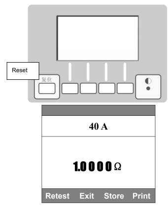
The display is dot matrix LCD screen, operating tips, measuring results, and function display of 4 function keys can be shown through it. The lower-left side is the reset key. When system halt appear or you want to exit from menu, pressing "Reset" key return to the initial state of the instrument; the lower-right side is contrast adjustment holes to adjust the LCD contrast.
