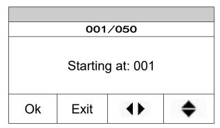
Before printing, you need to set the beginning and ending sequence number of data, use " • " key to switch sequence number, use " • " key to select digital, press "OK" key to confirm operation.
