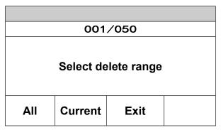
Press "All" key to delete all the stored data; press "current" key to delete the data currently appeared in your eyes; Press "Exit" key to return to the check interface.
