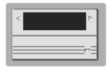
This instrument is equipped with a 16-line mini panel printer. It is easy to replace paper and ribbon and prints fast. It has a long service life and not need other maintenance and repair. The main power is on; the light on the lower-right corner of the printer will light indicating the printer in standby mode. During test or completed test pressing print key, you can print out the data.
