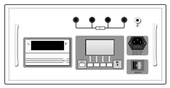
The panel layout as shown above consists of panel printer, LCD, keyboard, power outlet and power switch, output connecting terminal and ground terminal.
